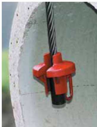
Drop pipe carrier lifting sling through hole in pipe. Align and insert Tea cup pipe carrier into lifting sling.
