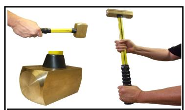
These BRASS HAMMERS are specifically designed for the precast concrete industry by *Blackthorn*. Pipe manufacturers & precasters have found this hammer to be a very durable tool when used to remove pallets. The soft material will not inflict damage to the pallet.
